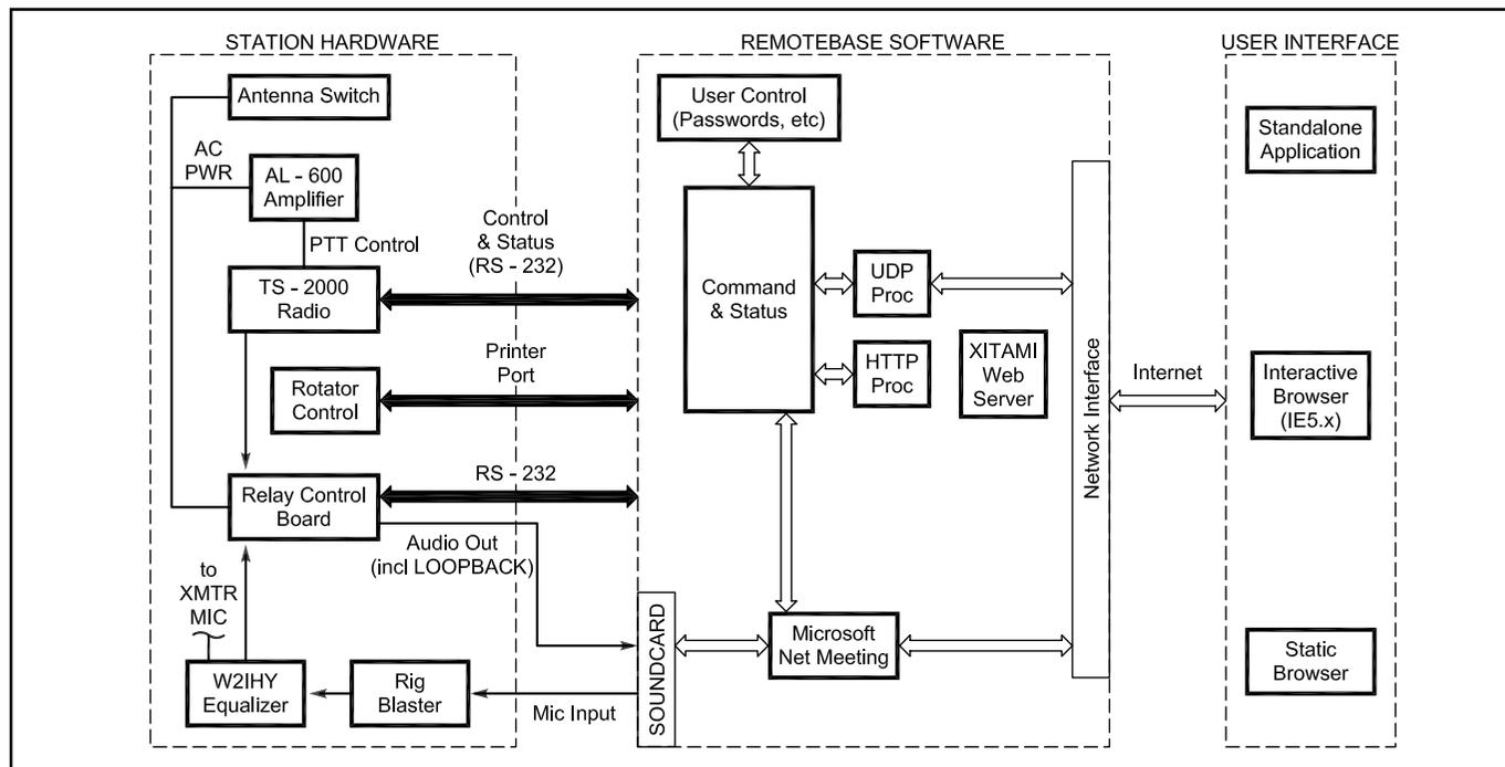
Figure 1—Block diagram of the W4MQ Internet remote base.
